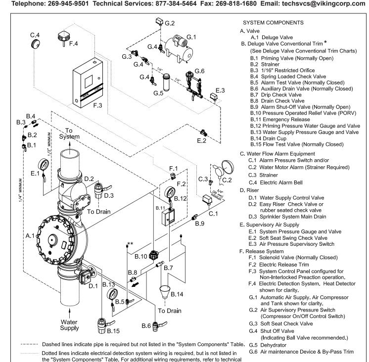
nipples. Viking Accessory Package for Conventional Deluge Valve Trim contains items B.2 through B.5, B7 through B.11, and B.14.
