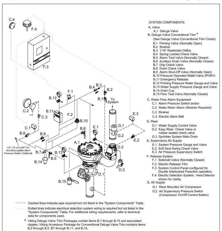
FIGURE 2: ANGLE DELUGE VALVE WITH RISER-MOUNTED COMPRESSOR (6" Valve Shown)
