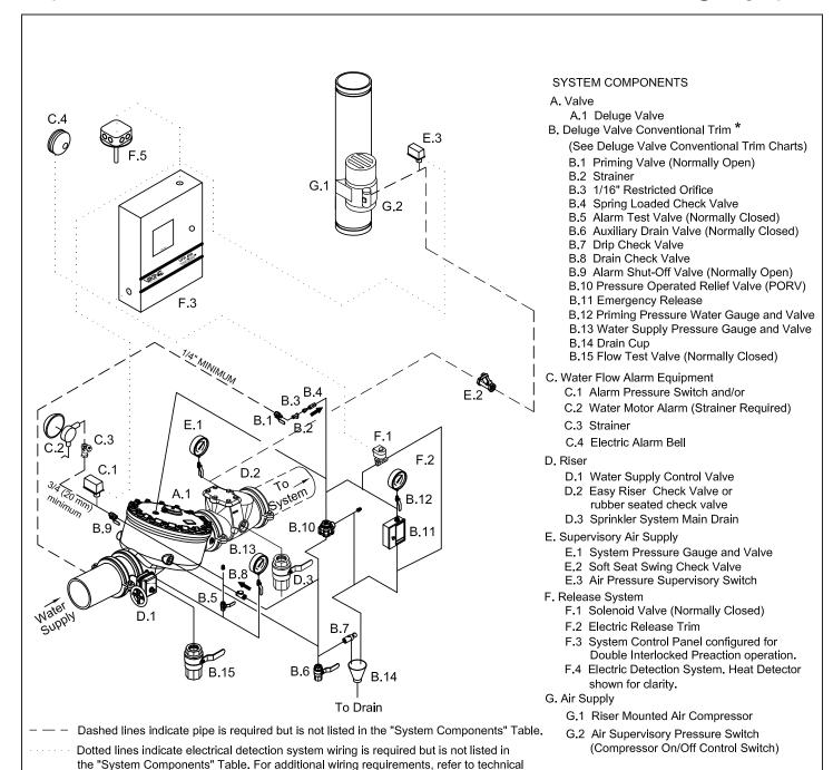
nipples. Viking Accessory Package for Conventional Deluge Valve Trim contains items B.2 through B.5, B7 through B.11, and B.14.
